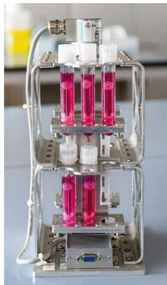
MagneTissue bioreactor with cultivated Schwann cells
