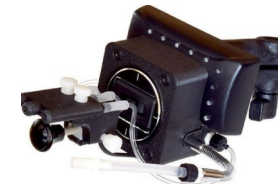
Quadstick mouth control with chin joystick, Deinhofer, Veigl(2025)
