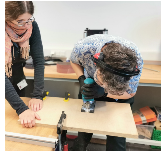
Figure 30: Cutting the inner case out of multiplex wood
