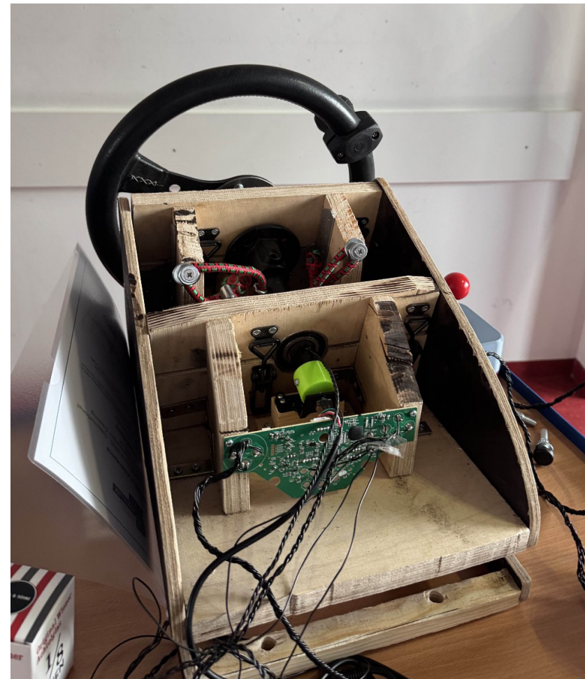
Figure 28: Steering Wheel with integrated electronics and sensors
