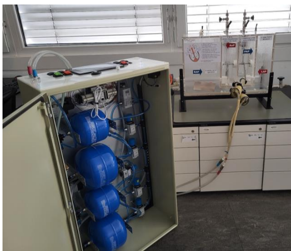
Figure 2: Current setup. Left: Pneumatic tanks and control. Right: Pneumatic pumps and heart mock-up
