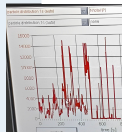
Figure 5: Results of particle distribution measurement with particle counter before filtering.
