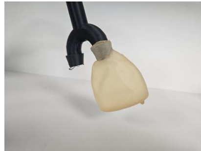
Fig. 5: Flexible lung lobe, attached to the U-connector
